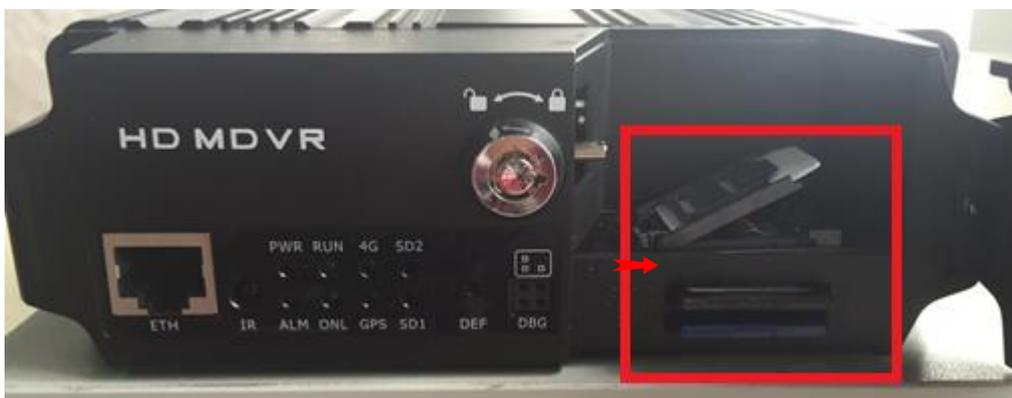
3. Close the shield and turn the device lock clockwise to locked.
