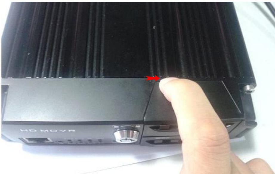
Figure 4.2\_2 insert SIM card and SD card
